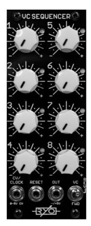
LjunggrenAudio RYO VC Sequencer: Compact 8-step Voltage Controlled Sequencer
